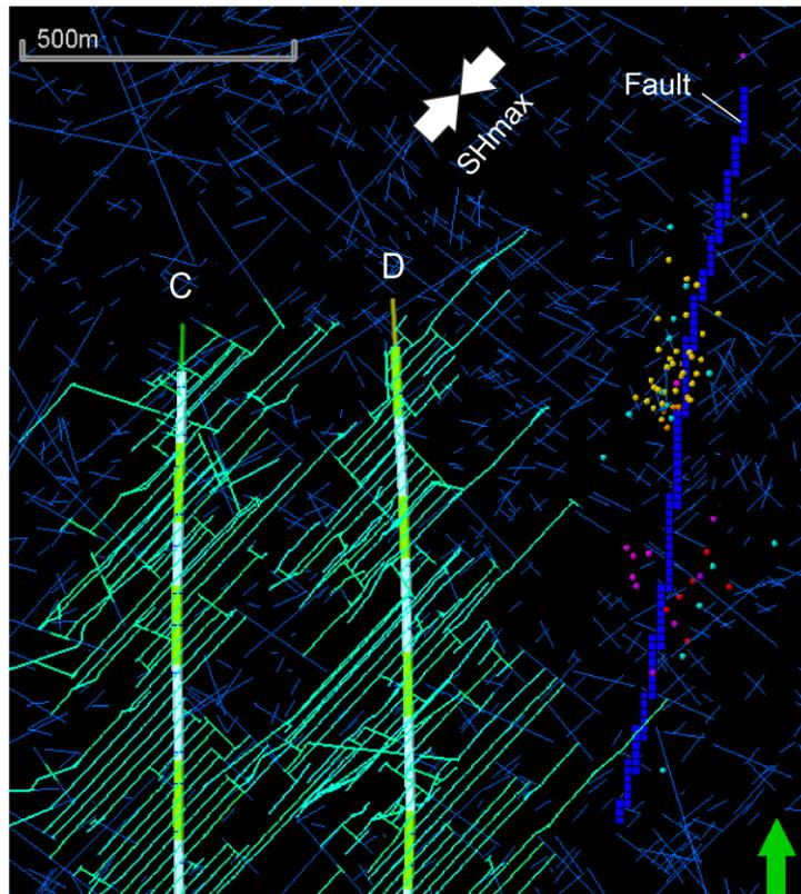
*Fig. 2. Simulated HFJs (green color) and NFJs (blue color) interaction during zipper fracturing of the Duvernay Formation in lateral wells C and D, after Konstantinovskaya et al. (2021). Fault is identified based on ant tracking attribute (Fig. 1a). The induced earthquakes are shown by time of occurrence on May 26 to June 14, 2015 (Fig. 1a).*
