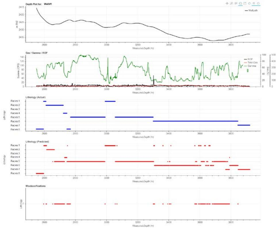
Figure 1: Dashboard displaying from top to bottom: the well path, gamma/gas/ROP data, Actual (blue) vs AI Predicted (red) lithofacies and misclassification
