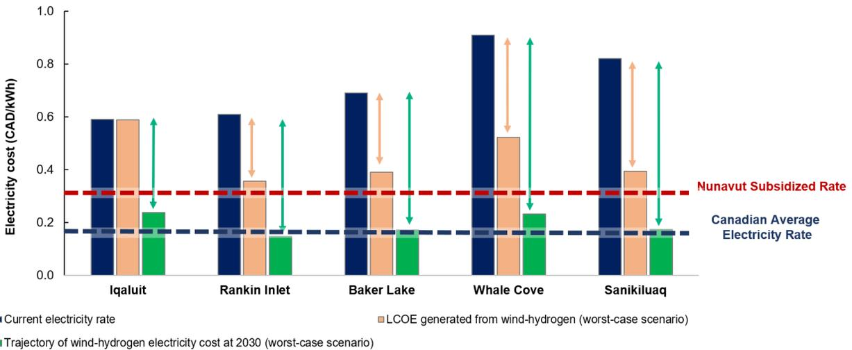
**Figure 2.** Model of five candidate communities for proposed wind-hydrogen coupled energy costs compared with existing diesel-generated electricity rates. Model inputs include the current diesel-only electricity rate (■), the wind-hydrogen levelized cost of electricity (■) and the projected wind-hydrogen cost in 2030 (■). Data sources: [9].
