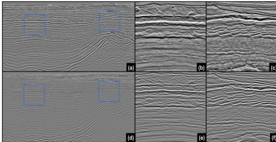
Figure 4: a) Reprocessing TTI KPSDM with b) left zoom section and c) right zoom section, compared to the d) legacy isotropic KPSTM stack with e) left zoom section and f) right zoom section. KPSDM stack stretched from depth to time for comparison.
