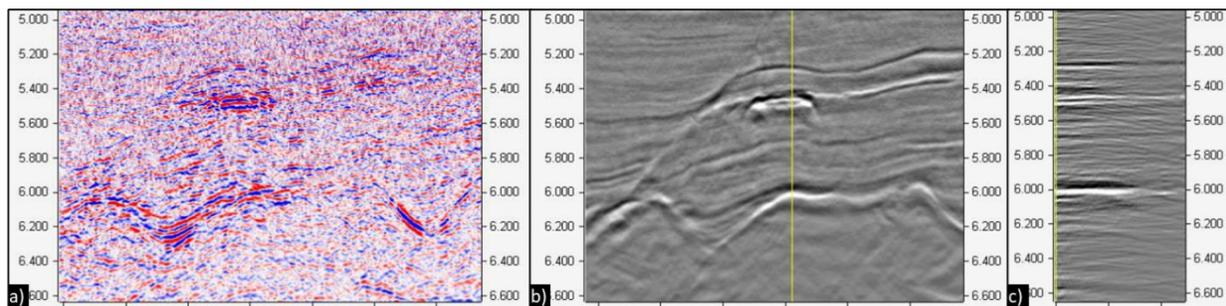
Figure 5: a) AVO Gradient with amplitude anomaly at appx. 5.5s b) Reprocessing TTI KPSDM stack stretched from depth to time c) Gathers corresponding to yellow line in b.
