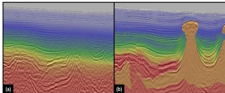
Figure 3:a) Single function initial p-velocity overlain on corresponding Kirchhoff Depth Migration (KDM) stack compared to b) final p-velocity overlain on corresponding KDM stack. 3:1 vertical exaggeration used to emphasize high-resolution detail.
