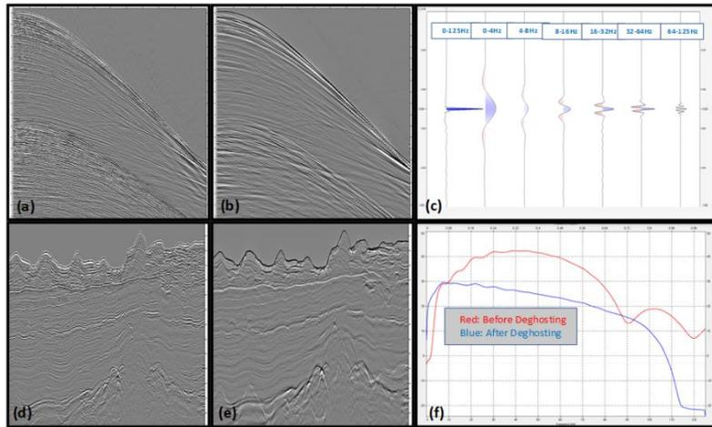
Figure 2:(a) Shot Gather before deghosting, (b) shot gather after deghosting, (c) WB wavelet and its filter panels, (d) stack before deghosting, (e) stack after deghosting and (f) amplitude spectrum comparison for the stack shown in (d) And (e).
