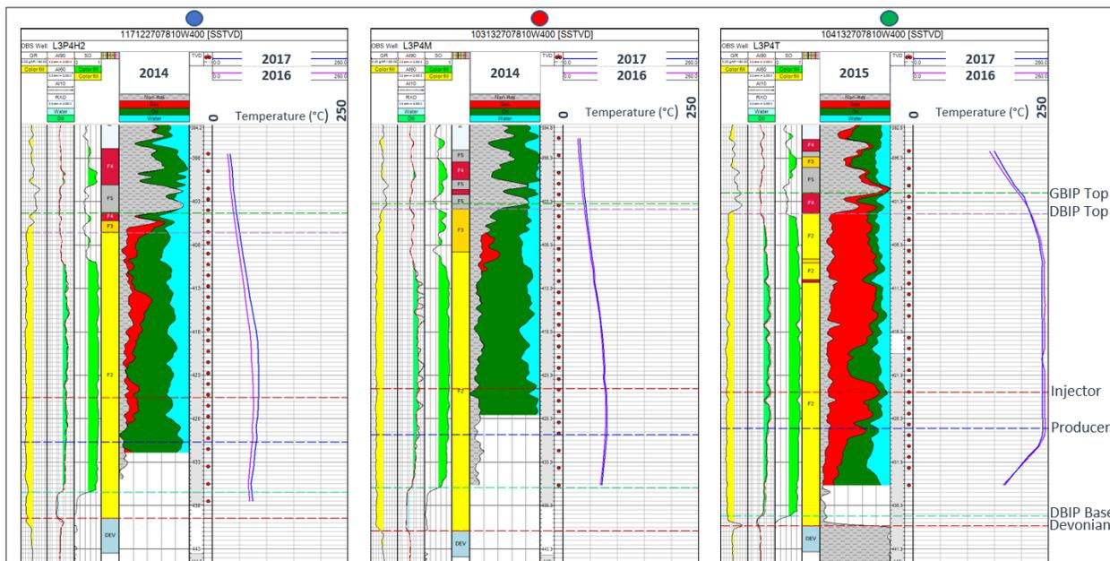
The heel to mid portion of the horizontal was relatively cool in 2017 and exhibited limited growth from 2016-2017. The toe portion of the well was at full steam temperature. The most recent 4D seismic survey prior to FCD installation was in 2014 showing the approximate elevation where bitumen is thermally mobilized.
