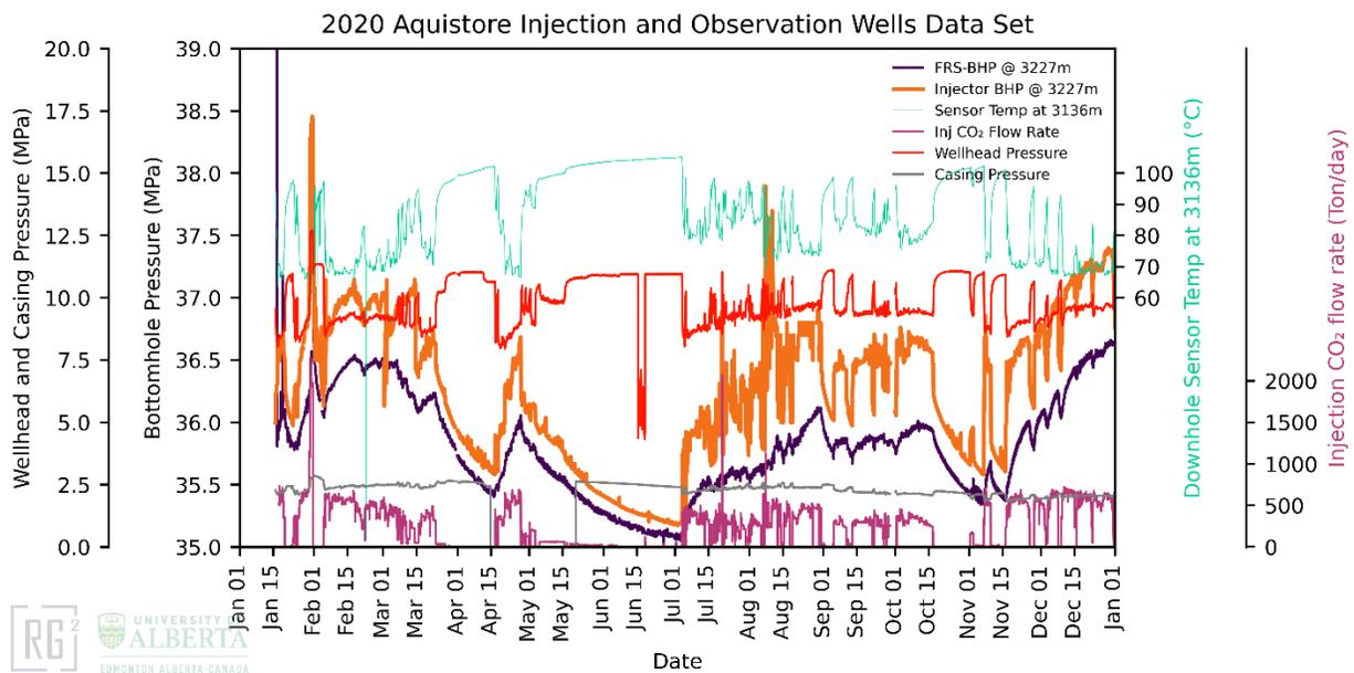
Figure 1 Aquistore Injector and observation well measurements during 2020.
