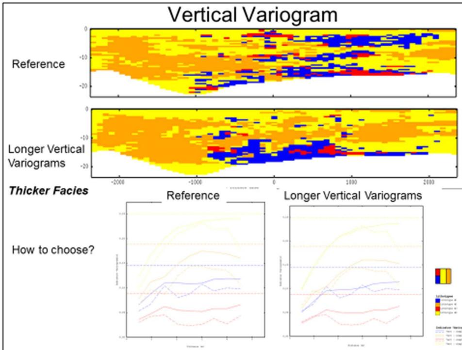
**Figure 2.** Choice of vertical variogram range based on fitting data has ambiguity. Honouring transition statistics in wells is an underutilized way to check model behavior and to optimize these parameters.
