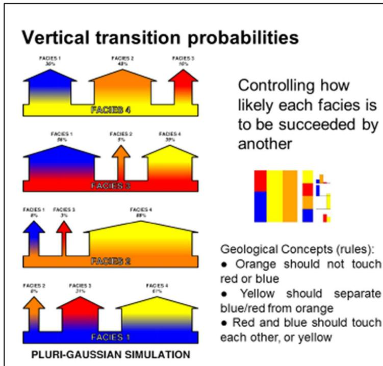
**Figure 1.** A slide that shows a graphical summary of vertical transition probabilities. The PGS approach directly gets the benefit of this information because this is an input to that workflow. Transition probabilities are a significant measure of continuity.
