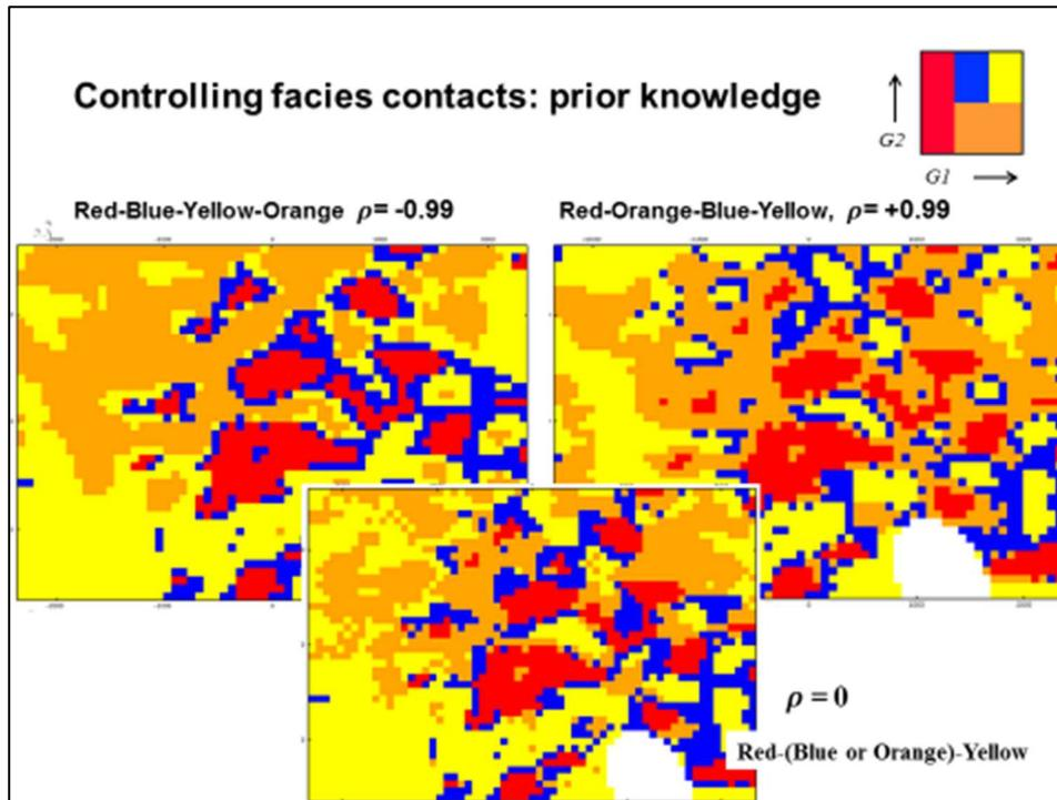
**Figure 3.** This example illustrates an extreme limit of geological patterns through use of the correlation of facies contacts. Based on geological understanding, controls can be imposed and numerically checked against facies stacking patterns in wells. Useful metrics (MSE, KLD) are to be discussed to help rank and choose key parameters to improve geological model verisimilitude.
