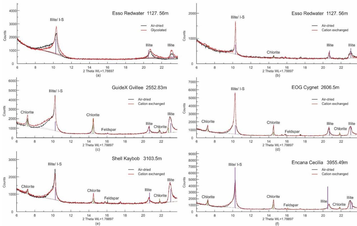
Figure 2 X-ray diffractograms of clay separates and whole rock of five representative samples.
