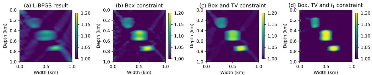
Figure 2: (a): Unconstrained result. (b): Inverse result with box constraint. (c): Inverse result with box and total variation constraint. (d): Inverse result with all three constraints.
