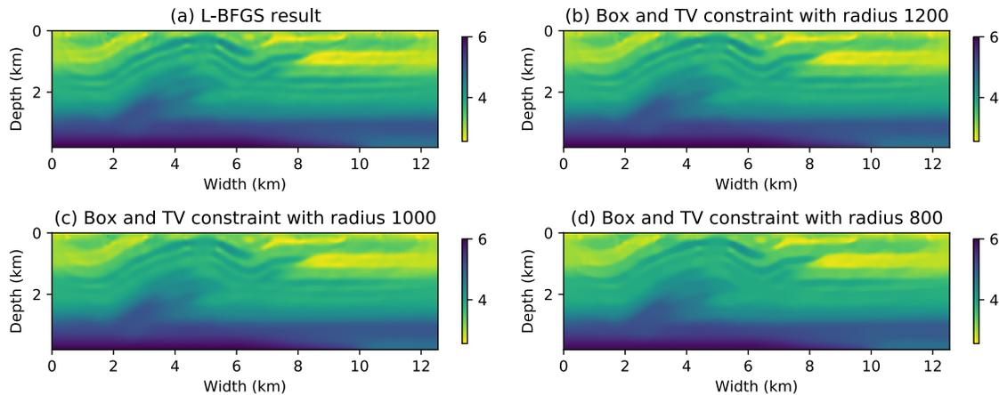
Figure 4: (a): Unconstrained result. (b), (c), (d): Inverse results with box and total variation constraints with different radius.
