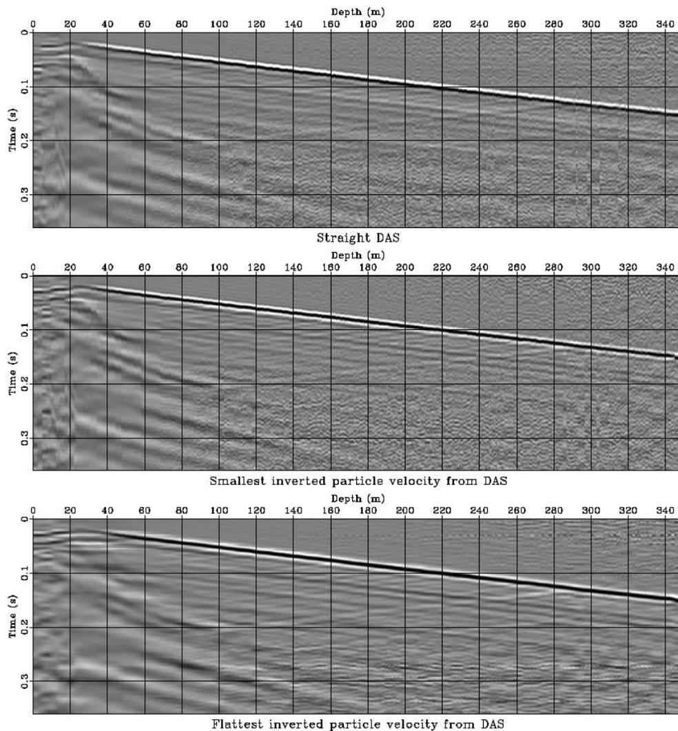
Figure 2: The top part is a straight fibre DAS vertical seismic profile shot gather from the Containment and Monitoring Institute Field Research Station (CaMI-FRS). The middle shows the vertical particle velocity inverted from the DAS data using the identity operator as regularization operator to obtain the smallest
