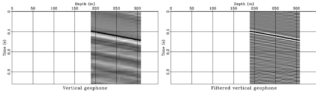
Figure 3: Vertical geophone shot gather corresponding the the DAS shot gather of Figure 2. Geophones are installed in the observation well from 191m to 306m depth every 5m. The left is the original data and the right is a 50Hz low cut filtered version.
