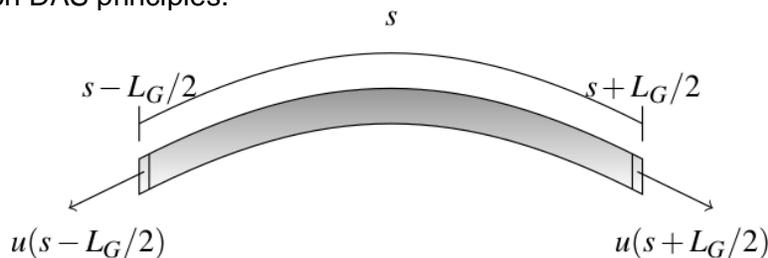
Figure 1: Displacements along a portion of fibre of length  $L_G$ , the gauge length, centred around point  $s$ . The total dilation or contraction of this fibre portion detected by the interferometer is the difference between the displacements  $u$  along the fibre at both ends.
