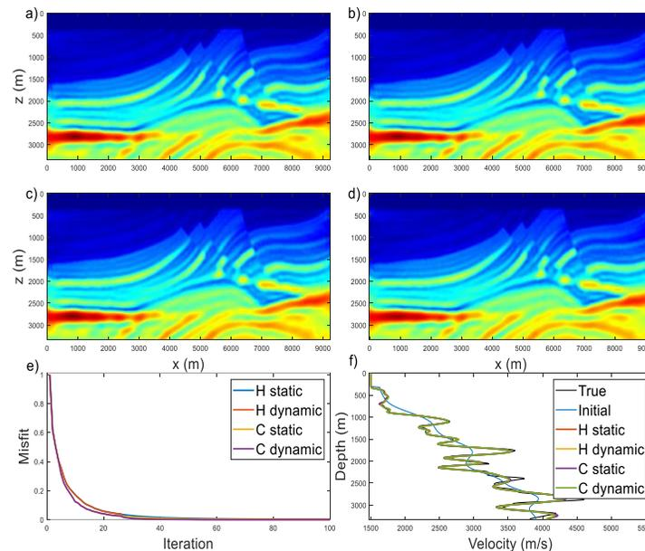
Figure 3: Comparison between dynamic and static encoding strategies: a) and b) are the inversion results by static amplitude encoding FWI using Hartley and cosine bases, respectively; c) and d) are the inversion results by dynamic amplitude encoding FWI using Hartley and cosine bases, respectively; e) is the comparison of misfit function versus iteration; f) is the comparison of vertical profile at the middle of the model.
