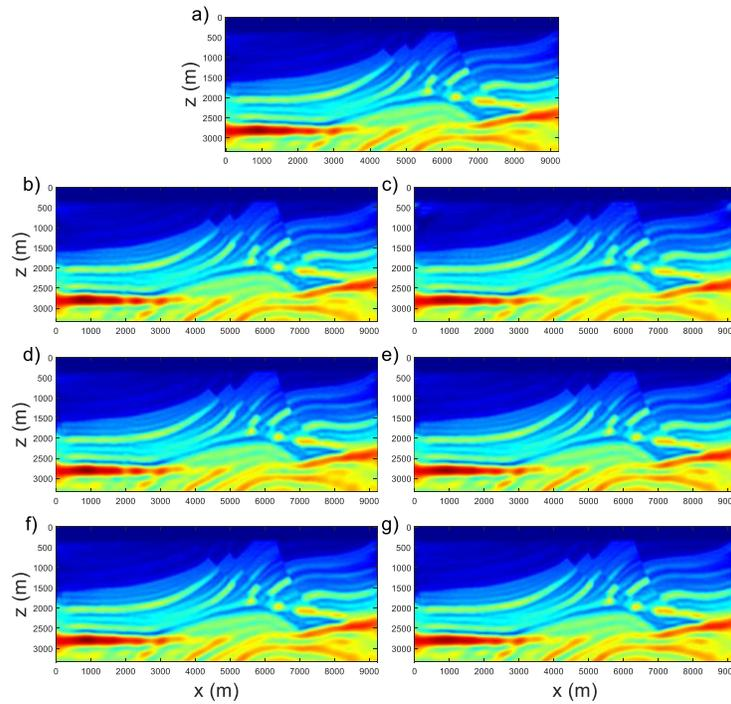
Figure 1. The updated velocity model after 100 iterations: a) by conventional FWI; b), d) and f) by amplitude-encoding FWI using Hartley basis with 7, 35 and 70 super-shots; c), e) and g) by amplitude-encoding FWI using cosine basis with 7, 35 and 70 super-shots.
