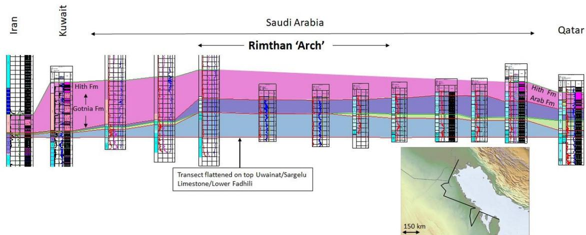
*Figure 1 – Regional log correlation highlighting the variation in facies and thicknesses of the stratigraphic packages between the Rimthan ‘Arch’ and adjacent Hanifa and Gotnia basins. Aggradation of the Callovian and Oxfordian carbonate in light blue. Early Kimmeridgian lowstand in light green. Early Kimmeridgian highstand in dark blue. Upper Kimmeridgian evaporitic sequences in pink.*
