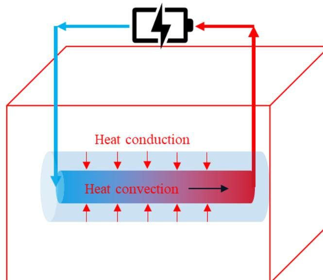
Figure 1. Schematic diagram of a closed-loop geothermal energy recovery system and its heat transfer mechanism. Colours represent working fluid temperatures ranging from cold (blue) to hot (red). The battery symbol reflects end heat usage (direct heat use and/or power generation).
