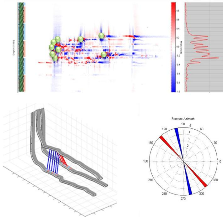
Figure 1 Top Image is a DAS waterfall display of fracture strain response from a neighboring well during a single stage completion. The summed strain is shown to the right. The bottom left image is the projected frac hits from two treated well. Bottom right image is the fracture azimuth of two completed wells.
