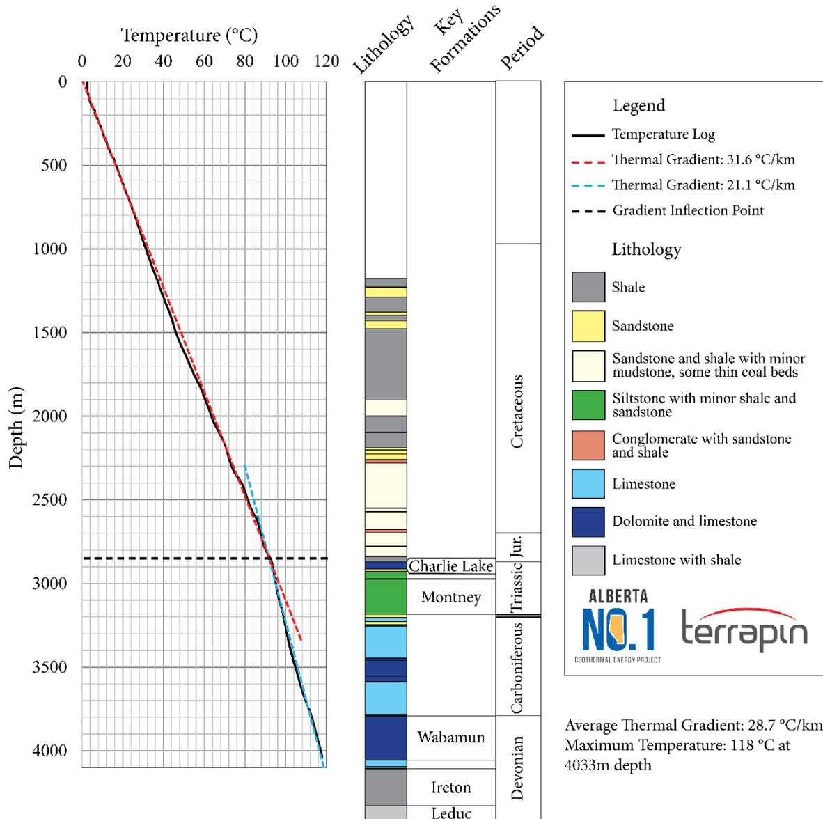
Figure 1. Temperature profile with depth and lithology log showing notable formations. The shift in thermal gradient occurs at the boundary between the Jurassic and Triassic, at the Charlie Lake Formation.
