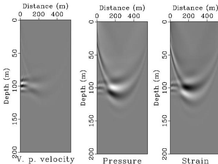
Figure 4: Synthetic data RTM. On the left is the usual vertical particle velocity RTM. On the middle is the pressure RTM obtained by using the imaging condition of equation 5, while on the right is the strain RTM created by using the imaging condition in equation 7.
