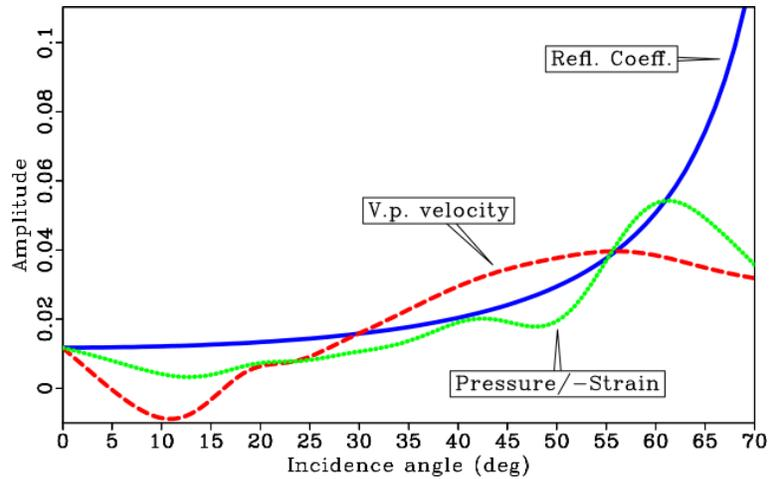
Figure 5: Theoretical geophone reflectivity and amplitudes extracted from the RTM images of Figure 4 at the reflector depth, 100m. The extracted amplitudes were stretched and shifted vertically to match the theoretical curve. Note that we are plotting the extracted amplitude strain with opposite polarity.
