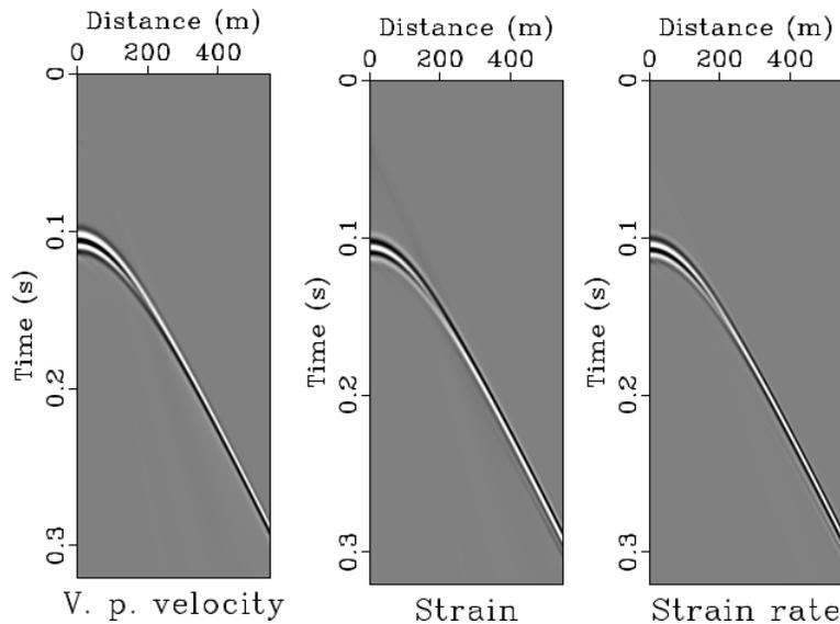
Figure 3: Synthetic DAS gathers. They were generated by using a finite difference scheme based on the system of equations 6. On the left is the vertical particle velocity,  $v_z$ , and in the centre is the vertical strain  $\epsilon_{zz}$ . The gather on the right is the strain rate and was created by deriving the gather on the middle. The first arrivals were muted.
