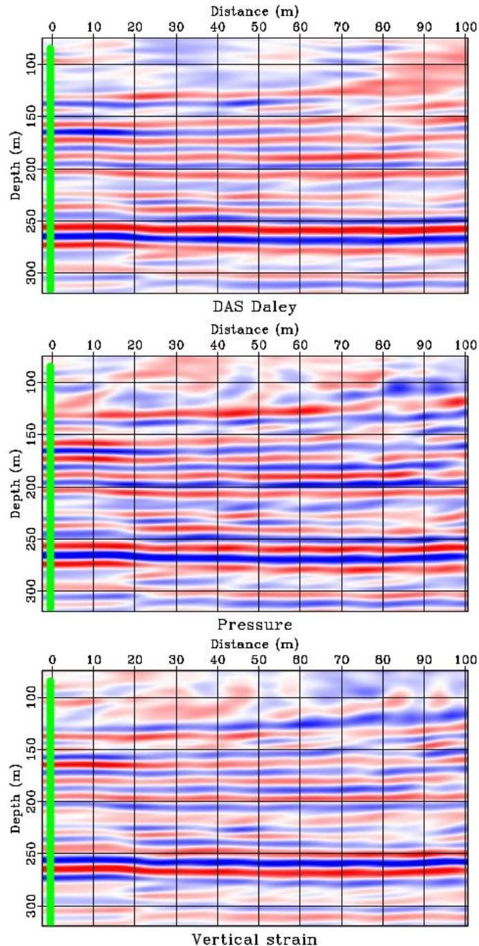
Figure 6: VSP DAS migrations with data from CaMI-FRS. Top shows the usual workflow that first turns the DAS data into geophone data by using the method of Daley et al. (2016) and then performs a particle velocity migration. Middle is the pressure RTM and bottom is the strain RTM.
