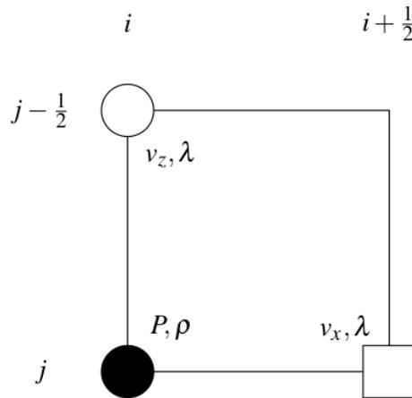
Figure 1: Location of the finite difference wavefields in the staggered grid. Pressure  $P$  and density  $\rho$  are at integer coordinates  $(i, j)$ , vertical particle velocity  $v_z$  is at coordinates  $(i, j - 1/2)$ , horizontal particle velocity  $v_x$  is at  $(i + 1/2, j)$  and Lamé parameter  $\lambda$  is defined at both  $(i, j - 1/2)$  and  $(i + 1/2, j)$ .
