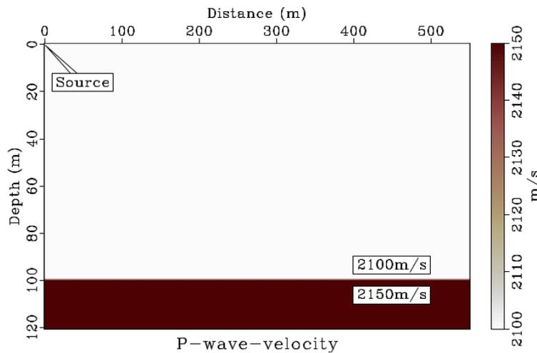
Figure 2: Synthetic experiment velocity model. The velocities follow Chattopadhyay and McMechan (2008) to obtain a range of precritical reflection angles up to  $77^\circ$ . The source is located at the top left corner and the DAS fibre along the surface.
