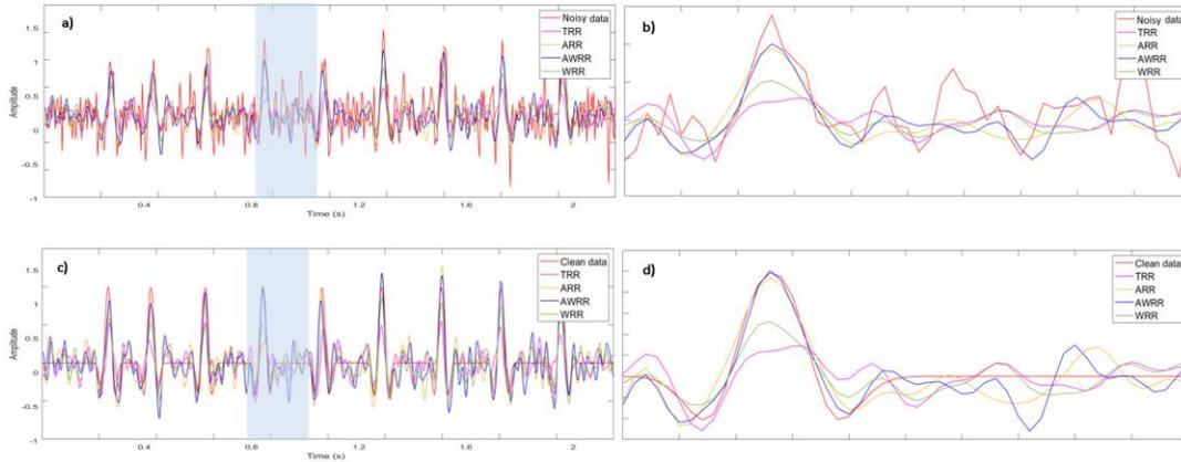
Figure 2: Amplitude comparison. (a) Comparison in the whole trace for the rank-reduction methods with the noisy data. (b) Zoomed area of the transparent blue window. (c) Comparison in the whole trace for the rank-reduction methods with the clean data. (d) Zoomed area of the transparent blue window.
