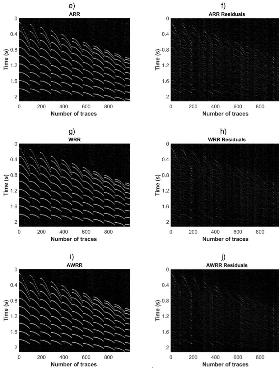
Figure 1: Applying different methods of rank reduction to a synthetic shot gather. (a) Input data with snr 4 and 60 percent gaps, (b) complete and clean data, (c), (e), (g), and (i) interpolated data using TRR, ARR, WRR, AWRR method, respectively. (d), (f), (h), and (j) Interpolation error of TRR, ARR, WRR, AWRR, respectively.
