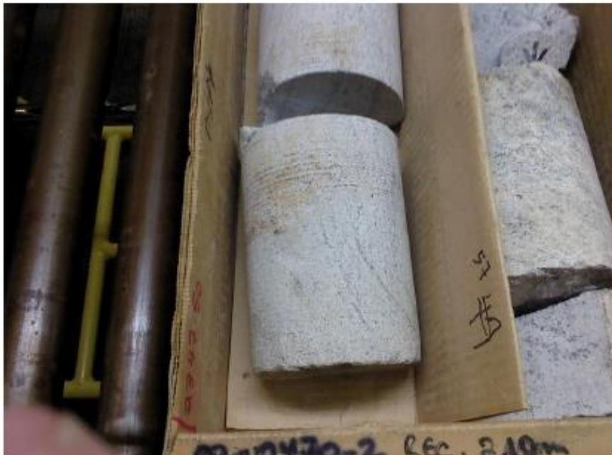
Fig. 3. Precambrian granite core from the deepest section of the Hunt well below 2300m (7,546 ft). The diameter of the core is 10cm (4 inches).
