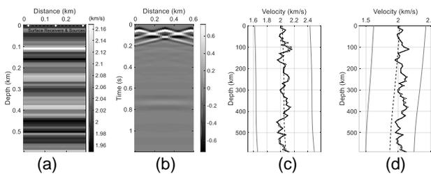
Figure 1: (a) True velocity model, and acquisition geometry. (b) Multisource observed data. (c) and (d) are, respectively, inverted results (dash-dot lines) using unbiased and biased initial models (dash lines). The solid lines are true models, the gray lines are bounds.
