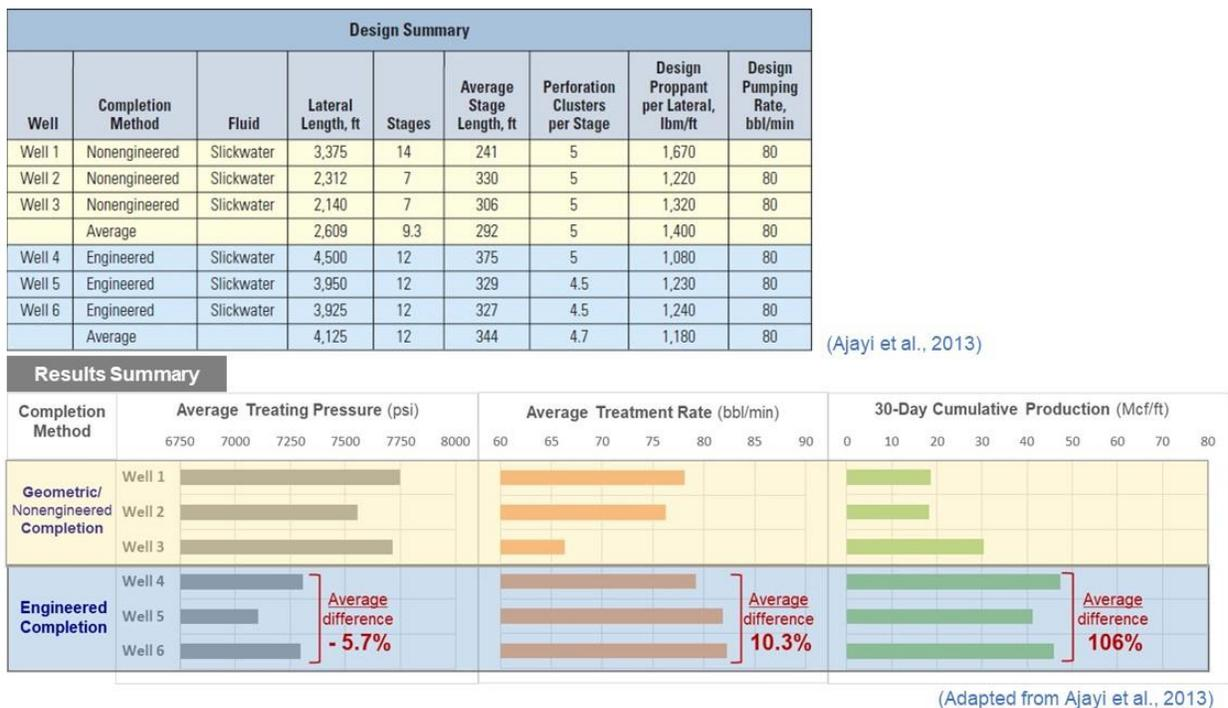
Figure 3 Nonengineered/geometric and engineered completions summary (Ajayi et al, 2013)
