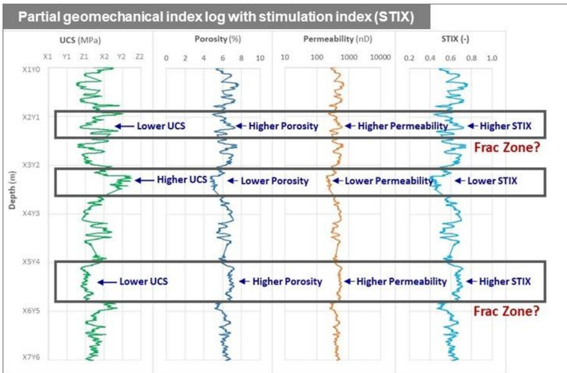
Figure 2 Summary results and geomechanical index log (partial) with STIX
