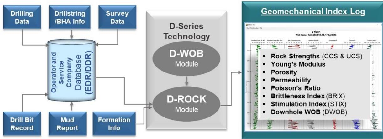
Figure 1 System overview of D-Series technology
