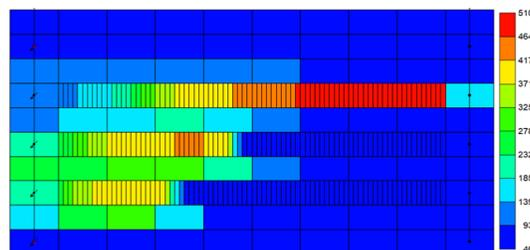
Figure 2 Effect of permeability in each layer on combustion front velocity
