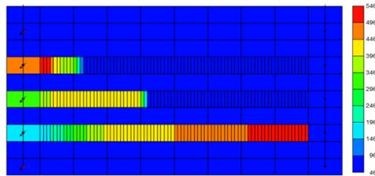
Figure 3 Effect of oil saturation in each layer on combustion front velocity
