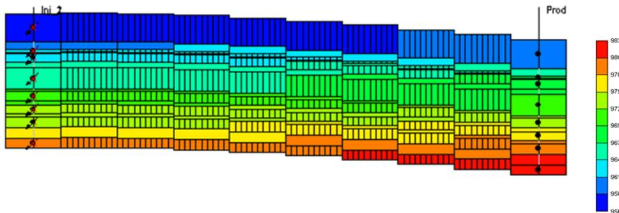
Figure 1 The simulation model of a multilayer heavy oil reservoir (grid top)
