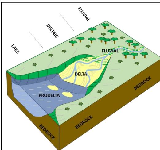
Figure 7. Sketch of Glenmore Reservoir showing a bayhead delta that only began forming following completion of the Glenmore Dam in 1935.
