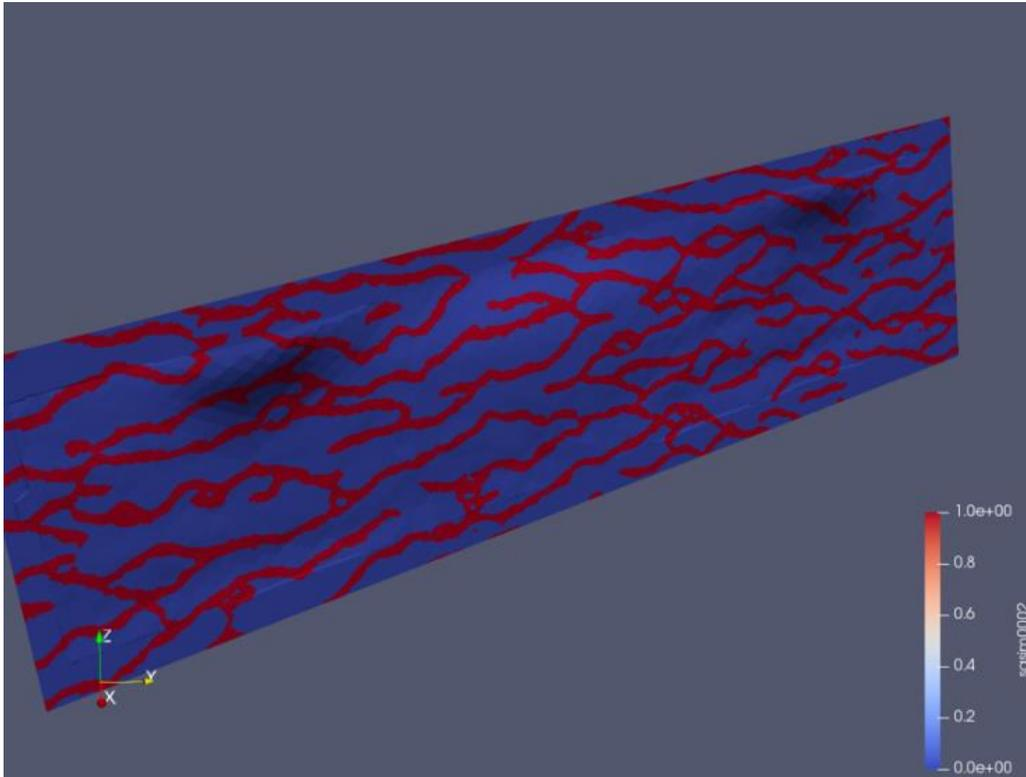
Figure 2: View of a simulated channel network within a single fracture zone.
