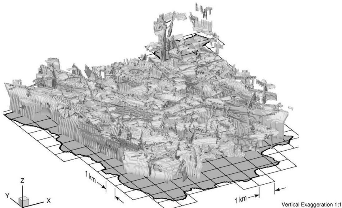
Figure 1: View of fracture zone network model mapped onto 3D groundwater model mesh.
