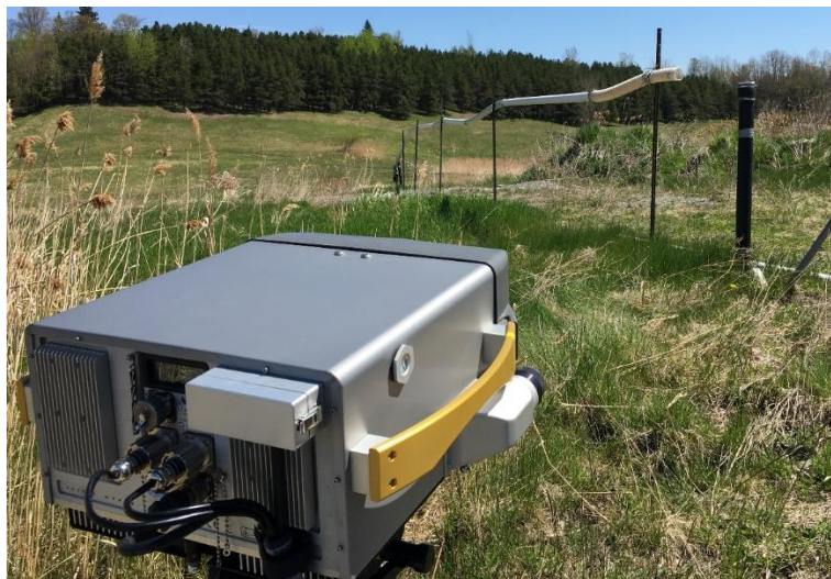
Figure 3: Hyper-Cam Methane focused on a sensing entry point of the methane collection
