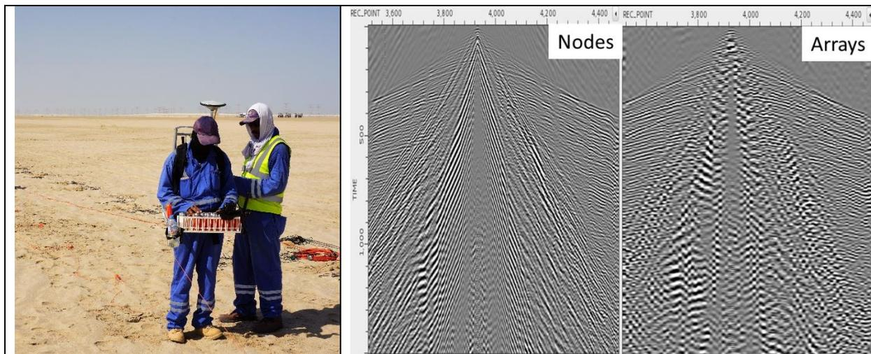
Figure 2 - 2D comparative field trial in desert environment (Ourabah et al, 2019). Left, deployment crew. Right, nodal system versus cable system shot gather.
