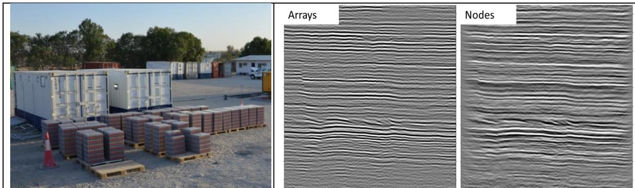
Figure 5 - Large scale field trial acquired by ADNOC in 2019 using 50,800 nodes (Ourabah and Crosby, 2020). Left, ~35,000 nodes on the ground in front of the charging and harvesting container and the cleaning container. Right, comparison of legacy data acquired with cable array system versus the new ultra-dense survey acquired with nodes.
