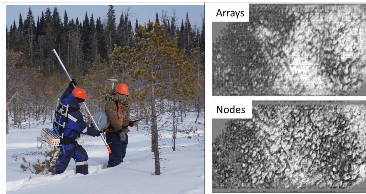
Figure 3 - 3D trial in Siberia with 8800 nodes (Brooks et al, 2018). Left, deployment crew. Right, time-slice comparison of PSTM fast-track processing of the nodal system and the cable system used in this survey.
