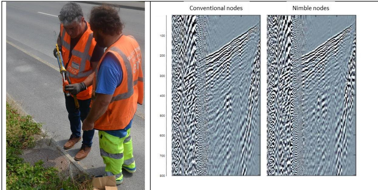
Figure 4 - Example of utilisation of the nodes in urban environment. Left, the crew testing deployment with silicon glue. Right, comparison of shot gathers of the two nodal systems used in this trial.
