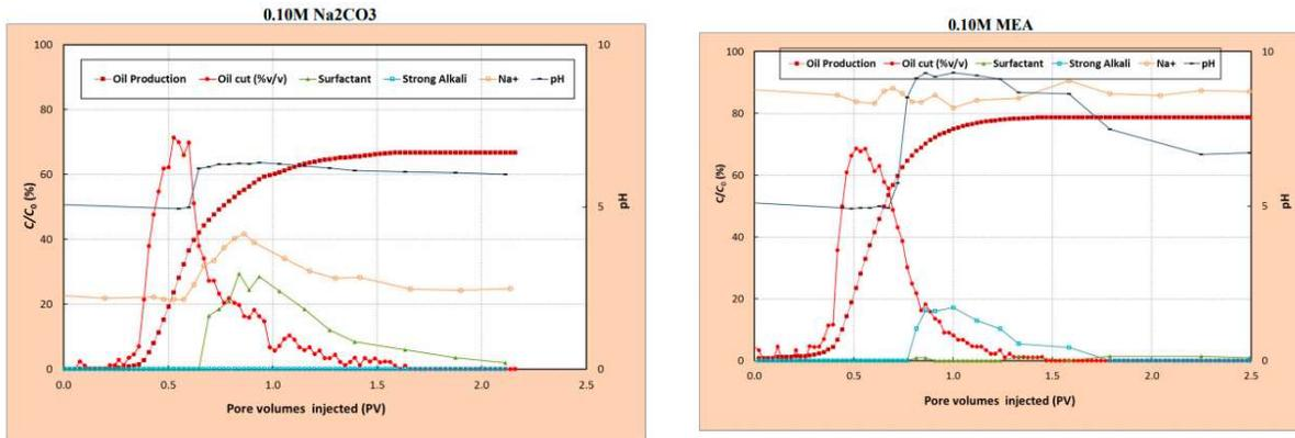
Fig. 4 from (4). Production plots for Boise core floods with 0.10M Na<sub>2</sub>CO<sub>3</sub> (left) and MEA (right).
