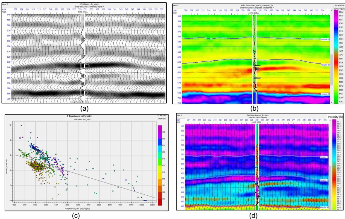
Figure 1. A seismic section from Alberta, where (a) is the stack, (b) is the P-impedance, (c) is the cross-plot of porosity versus impedance from the well over the gas sand, and (d) is the resulting of applying the regression line shown in (a) to the impedance section shown in Figure 1(b).
