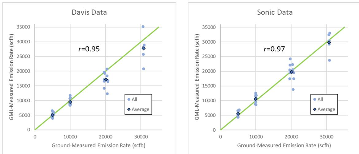
Figure 2 – Results of internal emissions detection testing
