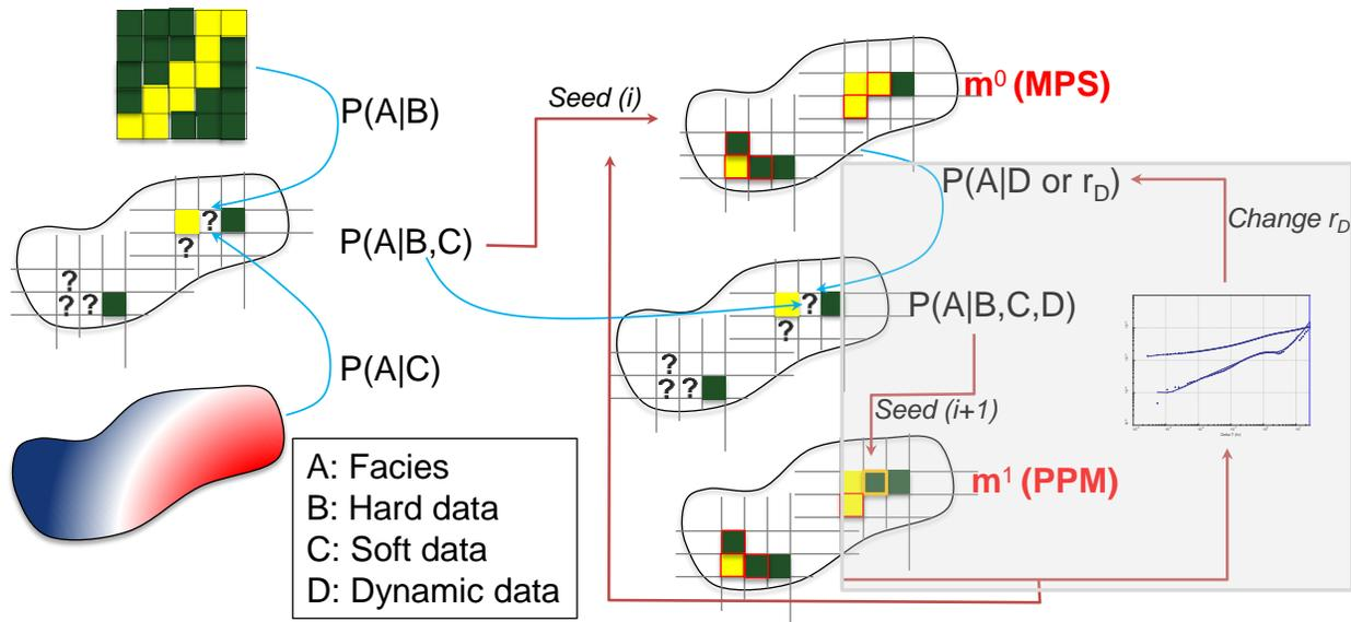
**Figure 1.** A general workflow for employing the PPM to calibrate the MPS realizations using the well test data. The realizations are generated sequentially by combining the probability of occurring the facies given the probability of available hard and soft data. Perturbation occurs in the probability space and the sequential sampling is used to sample from the local probabilities to generate facies realizations in the real space.
