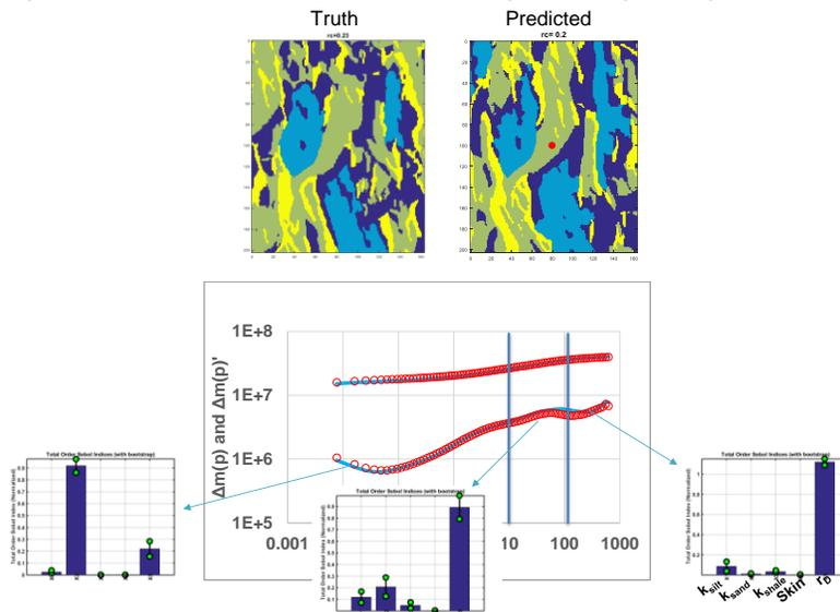
**Figure 2.** The results of calibration process. The predicted facies realization closely follows the truth case particularly in near wellbore areas (top). The simulated well test response also matches the signatures of the truth well test (bottom). The global sensitivity analyses for each segment of the well test signature (the histograms) show the importance of each variable on the well test signature changes with time.
