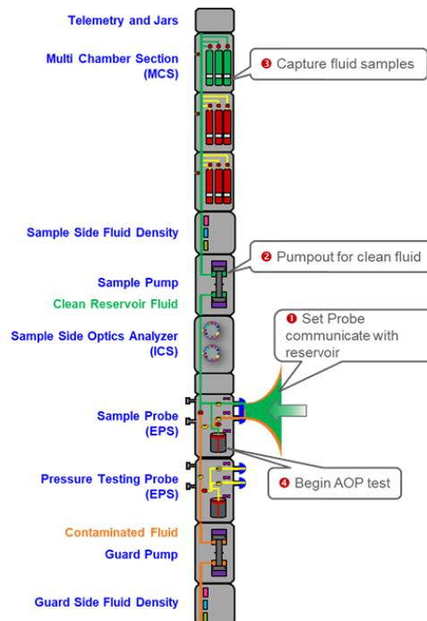
Figure 1: A wireline-conveyed formation tester was configured to perform downhole AOP measurements. The green cone and flowline signify clean oil, devoid of mud filtrate. The orange line signifies the mud filtrate contaminated fluid when configured for sampling by means of focused pump out. The numbered operations denote the sequence.
