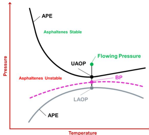
Figure 2: The asphaltene precipitation envelope (APE) denoting the stability regions of asphaltenes during production. The black line denotes the upper asphaltene boundary, while the lower gray line denotes the lower asphaltene boundary. The flowing pressure of the reservoir fluid is also marked, as it transitions from a stable asphaltenes region to an unstable region.
