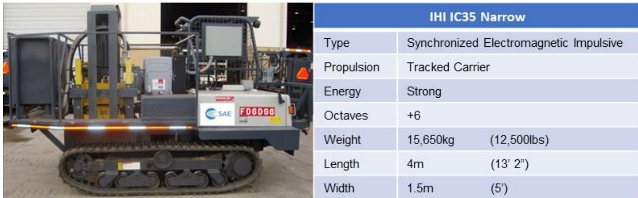
Figure 1: onSEIS™ Synchronized Electromagnetic Source
