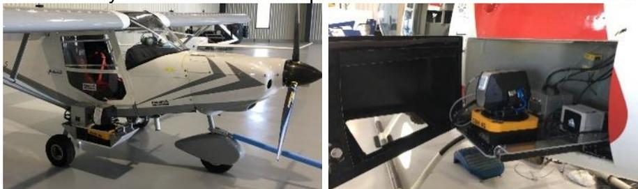
Figure 1. Example of integration of the Hyper-Cam Airborne Mini: (upper image) in an ARLA 600 from Asman Technology; (lower image) in a Bell 206 helicopter.
