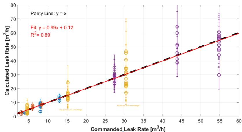
Figure 2. Parity chart of commanded methane leak rates and the corresponding reported calculated leak rate in m<sup>3</sup>/h. The  $y = x$  parity line indicates perfect quantification. Results show a close linear fit and good agreement between commanded and reported leak rates. The color of the data points indicates to which data collection campaign they belong.
