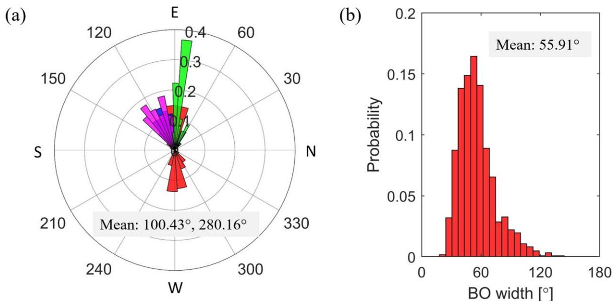
Figure 1 Statistics of breakout geometry at 1650-2000m. (a) Breakout orientations observed from UBI and caliper logs. Red, blue, magenta, and green bars represent the breakout orientation observed from UBI logs in 2013 and caliper logs in UBI PPC 2013, DSI PPC 2013 and Dipmeter 2011 respectively. (b) Breakout widths observed from UBI logs.
