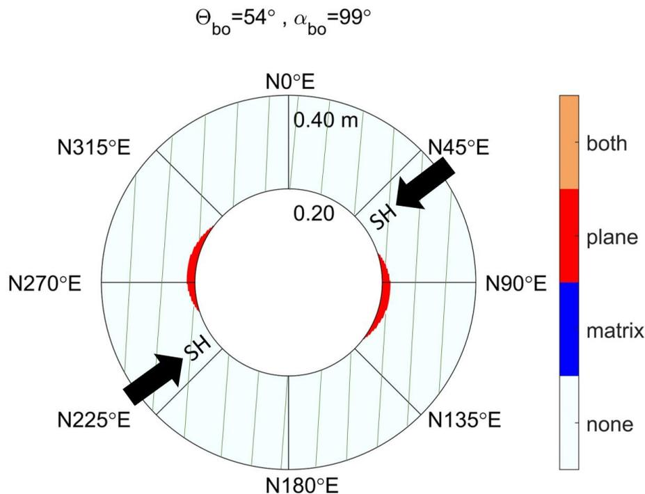
Figure 3 Modeled failure pattern. Parallel solid green lines represent the strike direction of the foliation planes. Light blue, dark blue, red, and orange areas represent no failure, failure only in the rock matrix, failure only in the weak plane and failure in both the rock matrix and the weak plane respectively. Two numbers at the top represent the breakout width  $\Theta_{bo}$  and azimuth  $\alpha_{bo}$  respectively.
