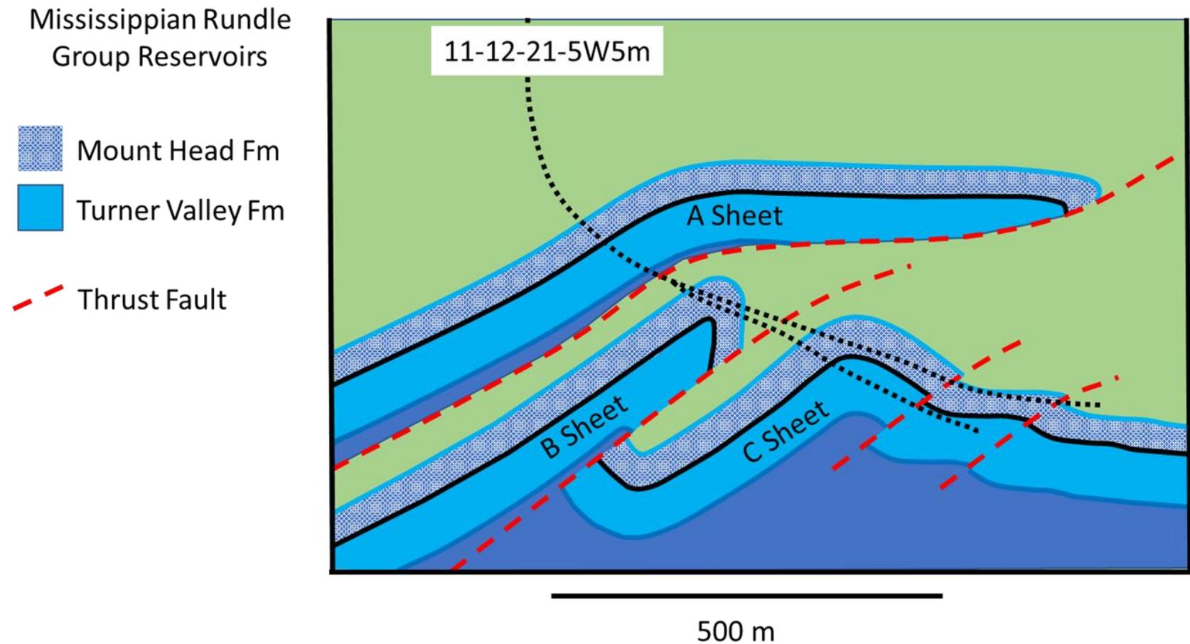
Figure 2. A generalized cross section showing the boreholes in relation to structure.
