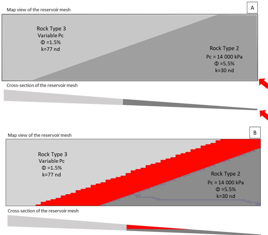
Figure 1: (A) Map view and cross-section (vertical exaggeration x5) of the reservoir mesh with the two different rock types. The rock type 2 in the deepest part of the reservoir has a capillary pressure set at 14,000 kPa. The red arrows indicate the injection point. (B) Example with gas accumulation below the seal formed by the rock type 3.
