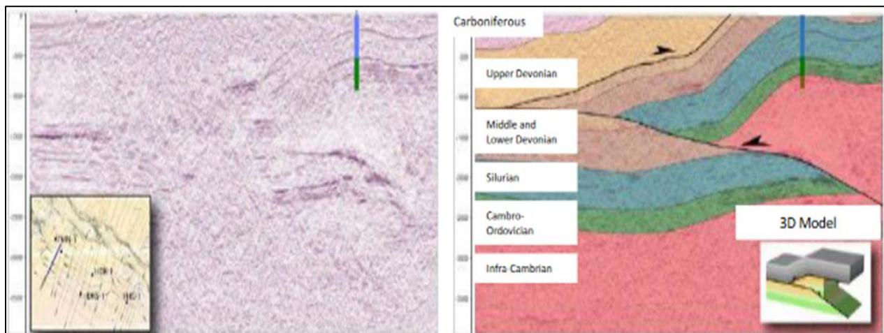
Figure 9: Overlapping deformation associated with a back-overlapping (triangular zone)
