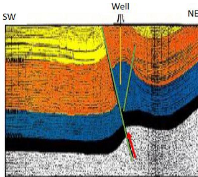
Figure 5: Structure anticlines against fault
