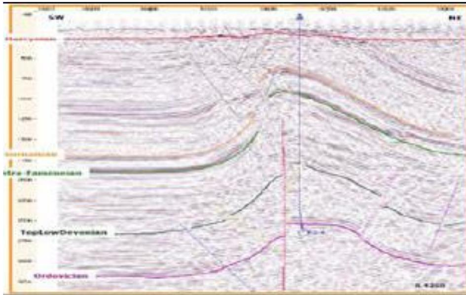
Figure 8: dextro-inverse faults and create sub anticlines parallel to the faults.
