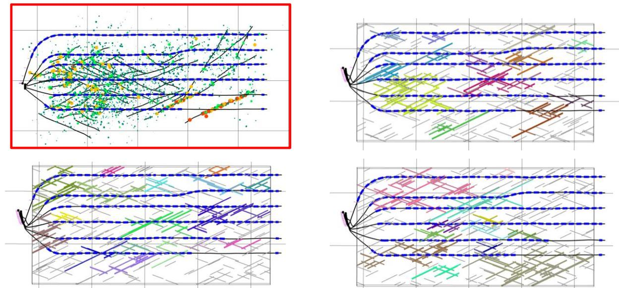
Figure 2: Example DFN model developed for a pad from observed events (top left), honouring the intensity of observed seismic lineaments, the size of observed lineaments and their orientation. Cluster analysis of the DFN shows patchy connectivity, explaining why limited higher magnitude seismicity occurs on a pad. The three other images represent 3 equi-probable structural realisations of the interpreted seismic lineaments (top left).
