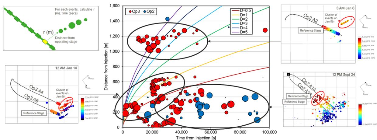
Figure 1: Examples of distance-time plots for a number of induced events. The coloured lines represent diffusivity curves for given values in the formula  $Distance = \sqrt{4\pi \cdot Dt}$  where  $D$  = diffusivity and  $t$  = time of flight
