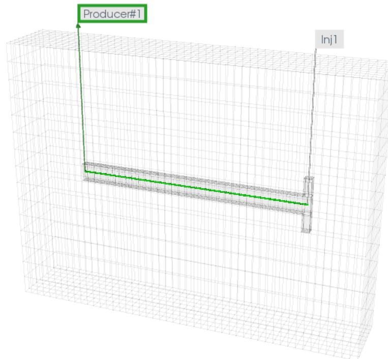
Figure 1. Schematic diagram of repurposing horizontal wellbore to the open-loop geothermal system by adding an additional injection well.
