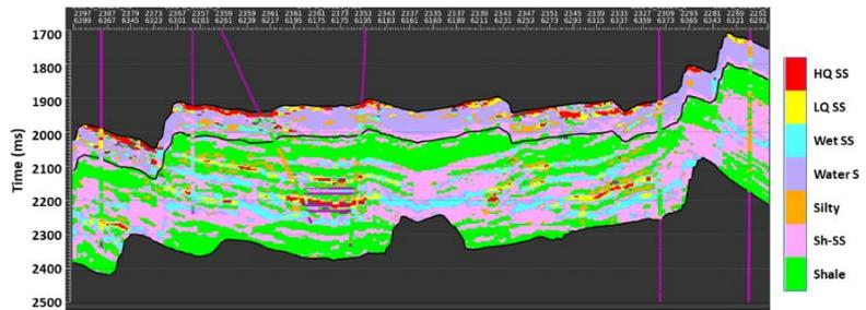
Figure 2: Most-probable facies from the Bayesian inference process described in Stage 2. The inputs were P Impedance and Vp/Vs from inversion.
