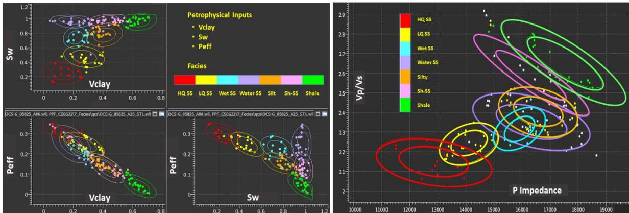
Figure 1: The left figure shows the petrophysical facies design from Sw, Vclay and effective porosity. Pdfs have been constructed corresponding to the seven facies. The first two standard deviations are shown. There is good separation of the facies types. On the right, the same facies have been shown in the elastic domain of P Impedance and Vp/Vs. The separation is not as good here but still enough to identify the facies end members.
