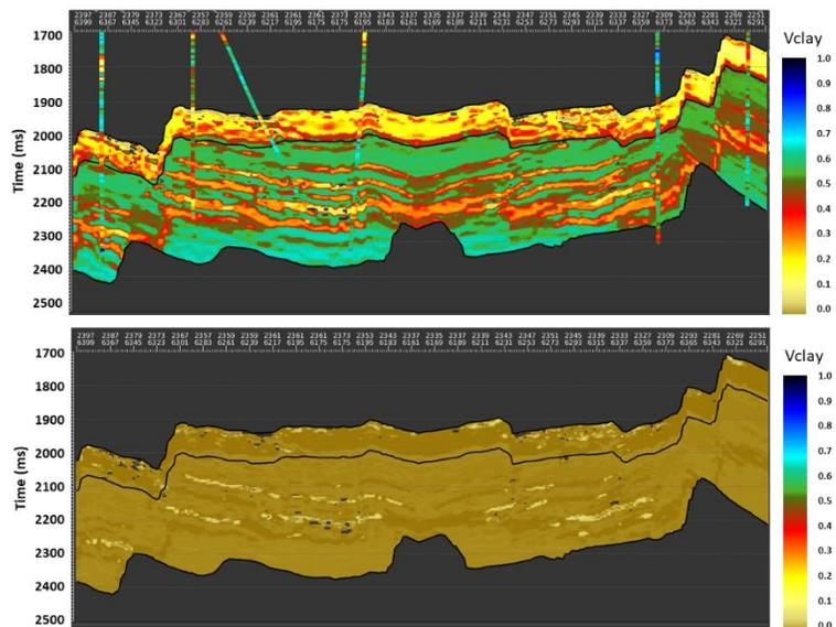
Figure 4: The upper panel shows the estimated Vclay from facies-driven modelling. Vclay logs have been overlain. The lower panel is the estimated standard deviation in Vclay from a set of facies probability assumptions. The possible range of the facies probabilities was estimated for each facies separately from the standard deviations of their Vclay PDFs. Note the variability in Vclay standard deviation across the figure.
