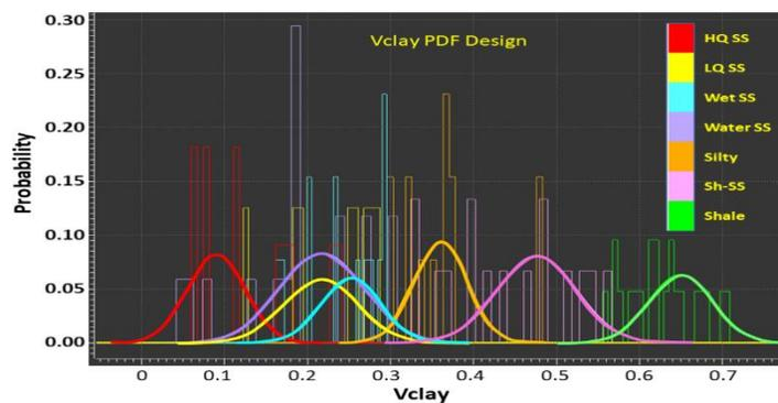
Figure 3: PDF design for Vclay estimation is shown in the figure. The background histograms are from log data.
