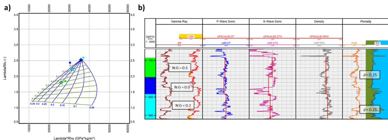
**Figure 2.** a) Rock-physics template with petrophysical values of N:G and porosity (stars) compared to the upscaled elastic properties (circles) showing close agreement. b) Log data showing petrophysical interpretations and upscaled elastic logs. The logs are upscaled into three zones.
