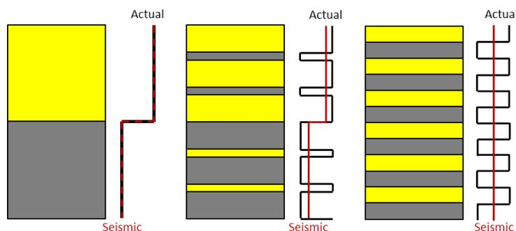
**Figure 1.** The observed elastic properties from seismic data match the properties of the individual layers when fully resolved (left). When thin layers, below seismic resolution, are introduced, the observed response is affected by a predictable amount (centre/right).
