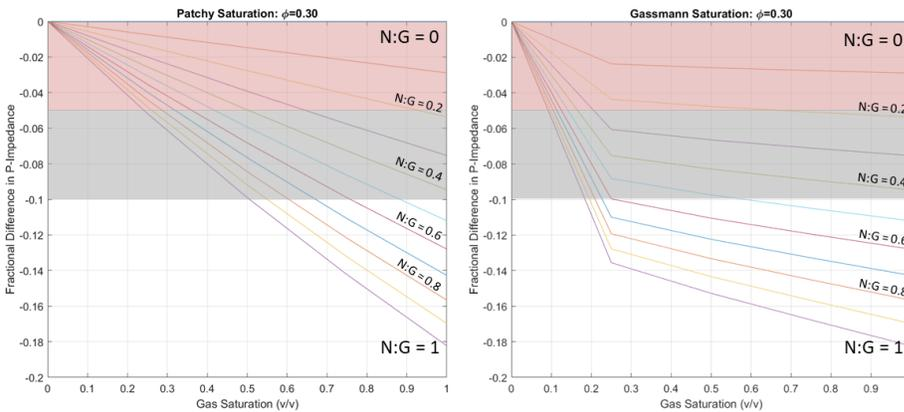
**Figure 3.** Difference in  $I_P$  from the wet case versus gas saturation. Each line corresponds to a different N:G, and the shaded areas indicate potential uncertainty in the inversion results.
