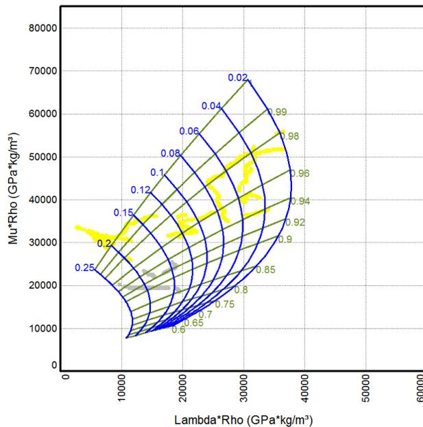
**Figure 5.** Rock-physics template for constant N:G and constant porosity along with upscaled log data. The log data in yellow has very few coal layers, while the data in grey has more. These proportions are consistent with the template lines of constant N:G (green).
