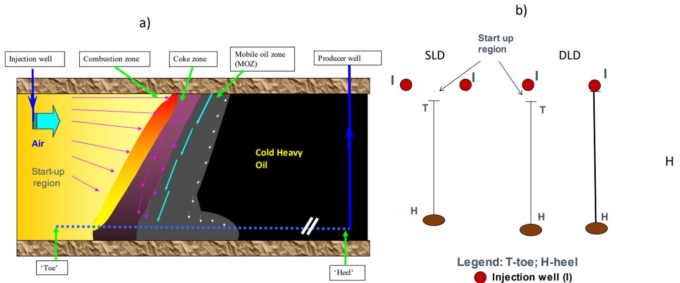
Figure 1: Schematics of THAI and its generalization for the case of ZERO start-up region (or without a start-up region). a) Schematics in vertical section ; b) Bird-eye view (view from above). DLD=direct line drive and SLD= staggered line drive
