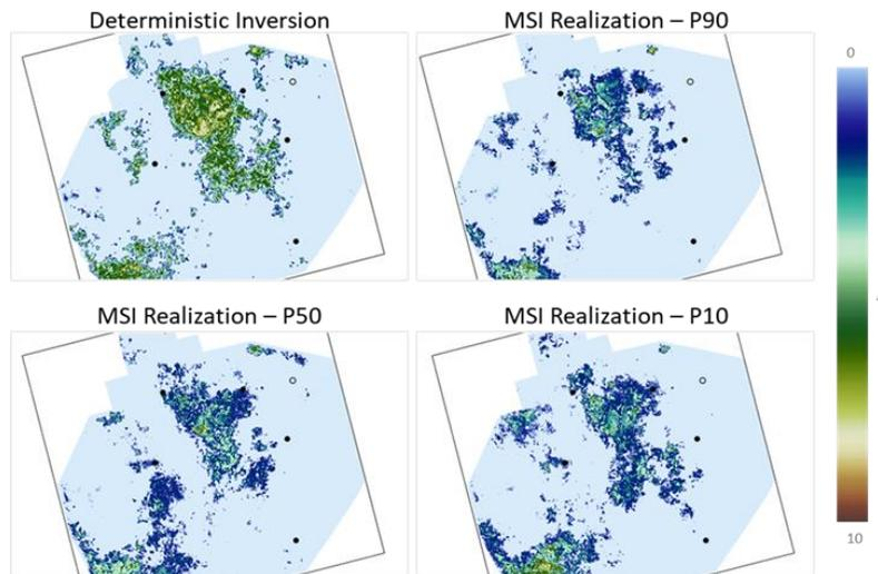
Figure 6. Comparison of thickness map of areas, with P-Impedance values above 40000 g\*ft/cc\*s in the target zone, generated from Deterministic inversion and p90, p50, p10 from MSI realizations. Thinner layers (as 8 feet, 2ms) can be detected and resolved in the MSI realizations volumes.
