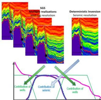
Figure 1. Modified Stochastic Inversion (MSI) schematic implementation in frequency domain.
