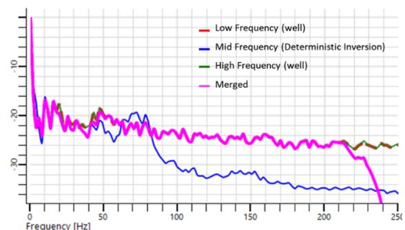
Figure 2. Modified Stochastic Inversion (MSI) output after the spectral merge (pink curve). Notice how more frequency content was added after the process. The blue curve represents the previous inversion volume spectrum.
