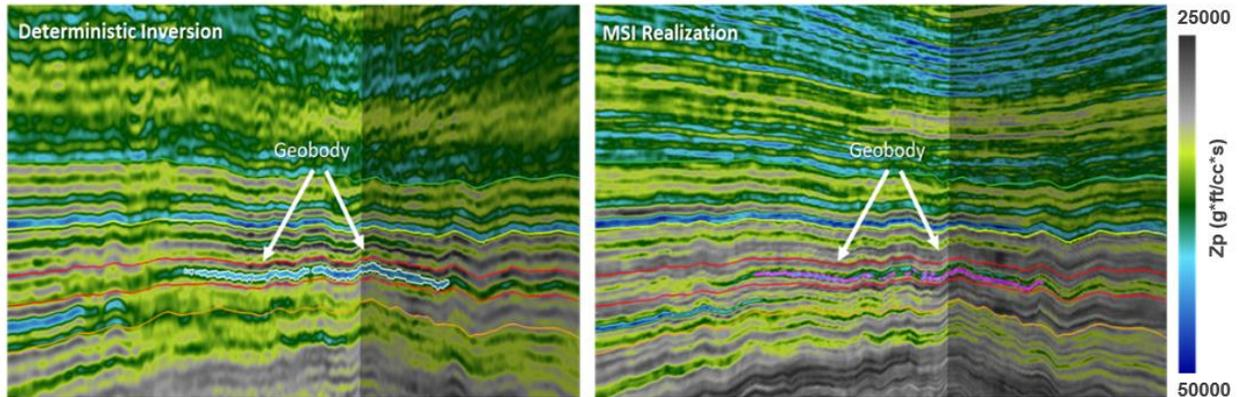
Figure 5. Cross-section through debris flow with geobodies extracted based on P-Impedance values above 40000 g\*ft/cc\*s, from the deterministic inversion volume (left) vs MSI realization P90 (right).
