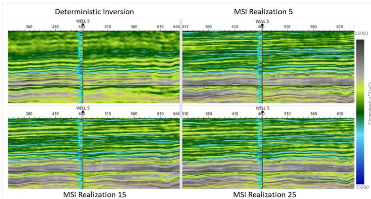
Figure 3. Comparison between Deterministic Inversion vs Realizations 5, 15 and 25 from Modified Stochastic Inversion (MSI) for P-Impedance. Notice the increase in detail in the reservoir and the variability between the realizations
