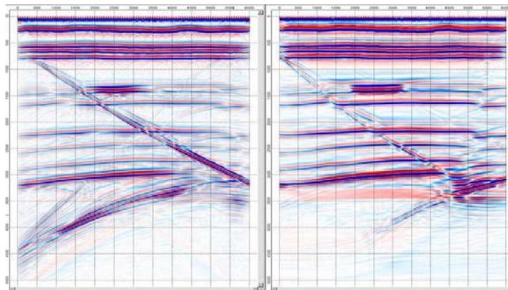
Fig. 11 Time CDP stacked section (left) and the corresponding post-stack time migration result (right).
