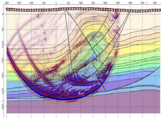
Fig. 6 Snapshot of the elastic wave field
