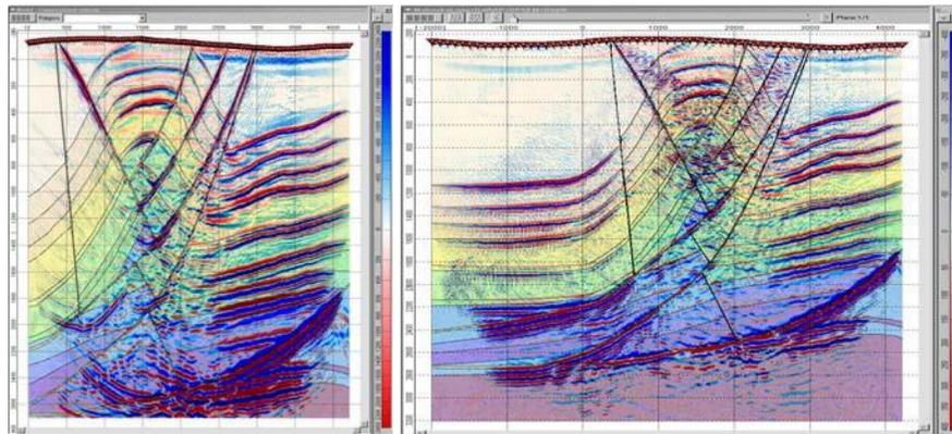
Fig. 8 Results of pre-stack depth migration in depth scale before and after a 2km expansion to the left and an increased in depth
