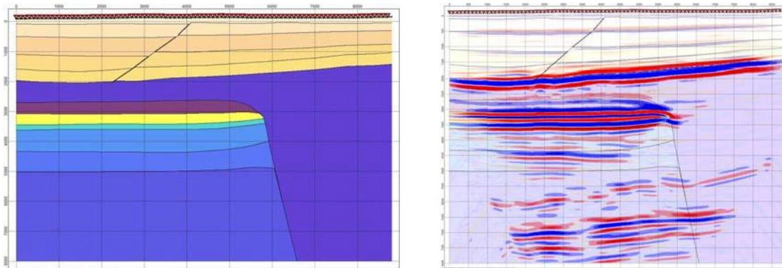
Fig. 9 Salt stock flank model and the results of pre-stack depth migration. Depth
