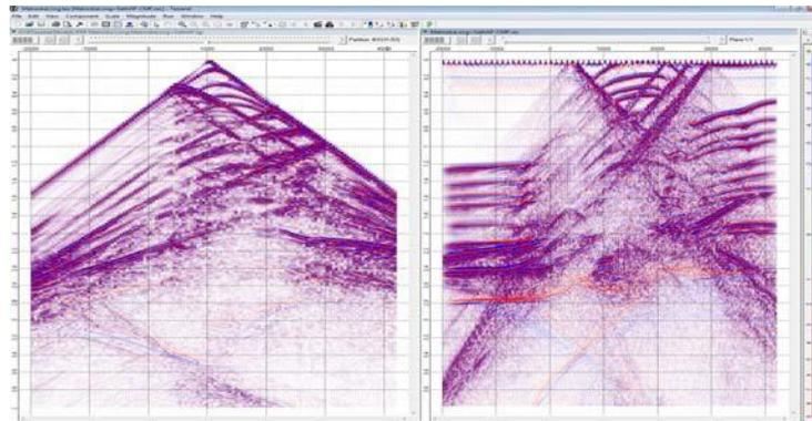
Fig. 7 A synthetic seismogram (left) and the CDP time section(right)
