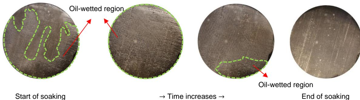
**Figure 1.** Open-end face of the core plug during the soaking stage of Test 1. Green dashed curves show the oil-wetted regions of the rock surface
