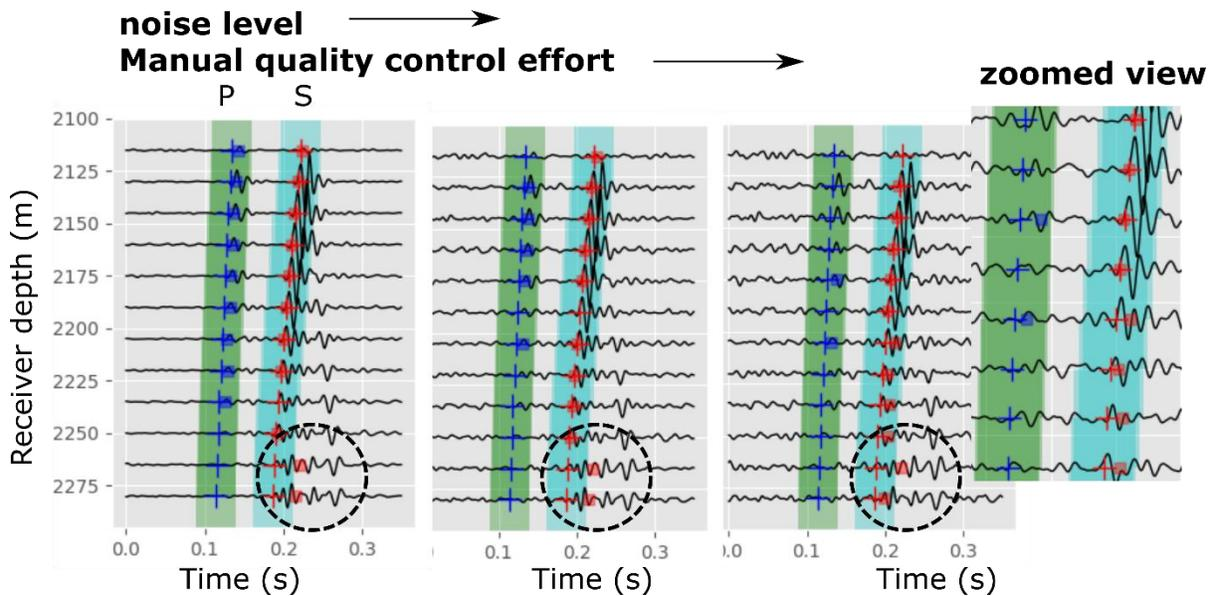
Figure 2: z-component of the waveforms from Figure 1 with the addition of Gaussian noise. Autopicking results from the fuzzy cmeans-AIC method are shown (squares) along with the modeled times (+) for comparison. The circles highlight the S-wave missed results.
