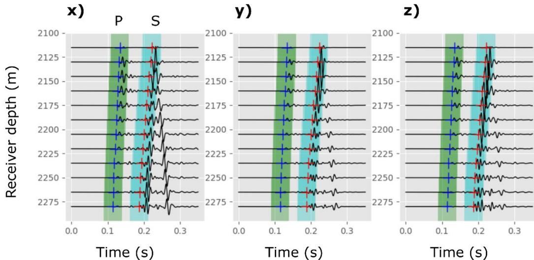
Figure 1: 3C waveform examples of a synthetic microseismic event. The time gates for semblance calculation as well as the modeled traveltimes for both P and S arrivals are shown.
