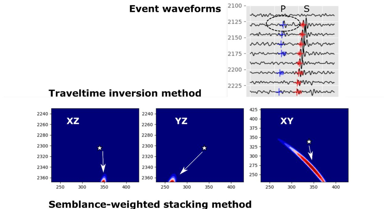
Figure 3: Example of the noisy waveforms for a microseismic event. The ellipse shows the arrival used as reference for the time gate. Manually corrected picks (+) are shown for comparison with the autopicking results (squares). The hypocenter locations determined using the traveltime inversion and semblance-weighted stacking approach is also shown. The true location is represented by the star sign.
