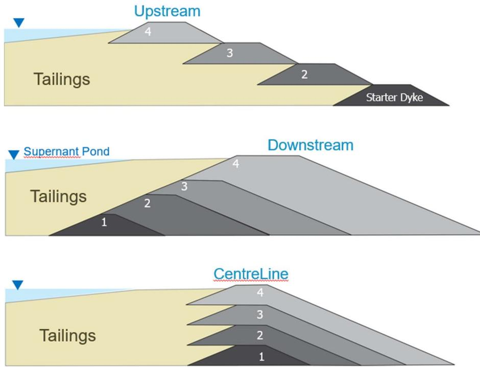
**Figure 2.** Schematic of sequentially raised tailings dam designs, where the name reflects the direction the crest moves relative to the starter dyke #1. The upstream version results in a dam crest constructed on a larger profile of fine tailings, which have low permeability and are susceptible to liquefaction, compared to that of the more desirable downstream and centreline designs.
