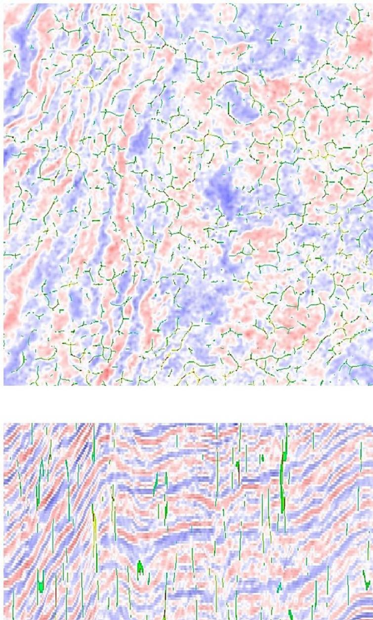
Figure 3. Seismic timeslice with embedded fracture attribute (top) and seismic section with embedded fracture attribute (bottom) [modified from Hawas et.al., 2018]
