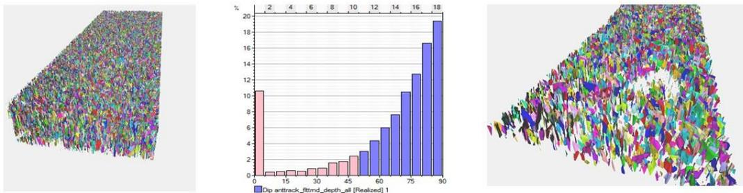
Figure 4. Extracted fracture patches (left); dip filtering of patches (middle); fracture patches truncated to reservoir limit (right). Modified from Hawas et.al, 2018.
