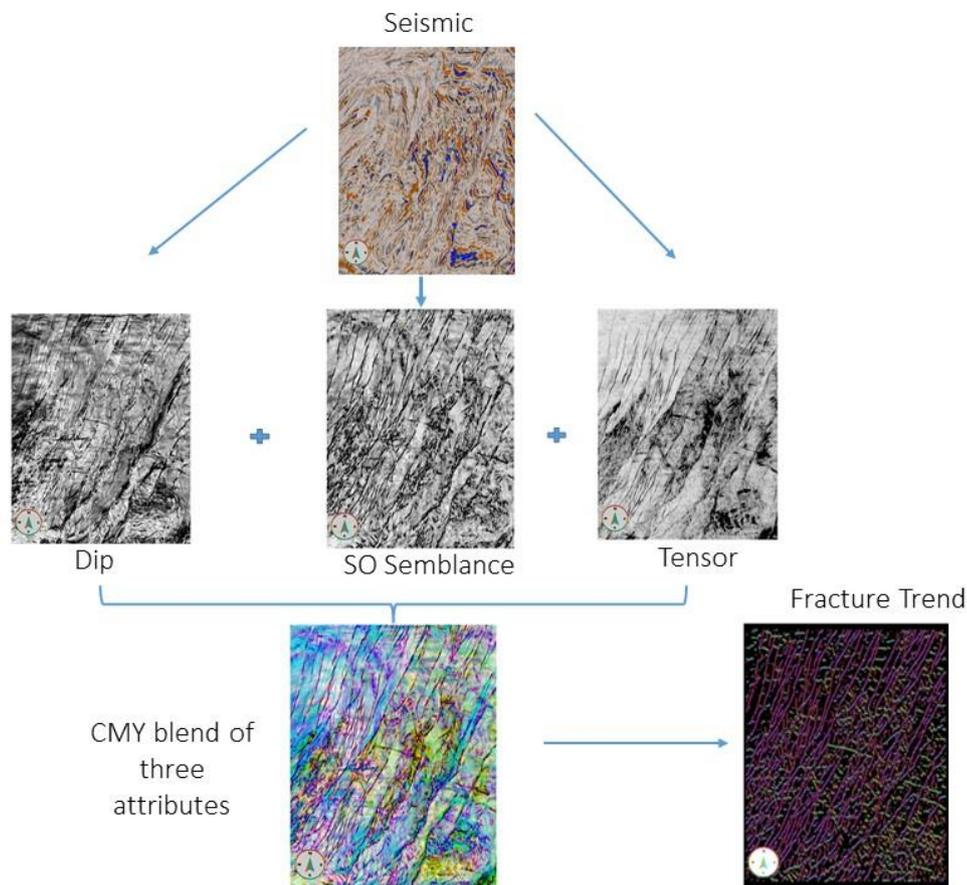
Figure 2. Creation of fracture attribute from three independent attributes: dip, semblance, and tensor.
