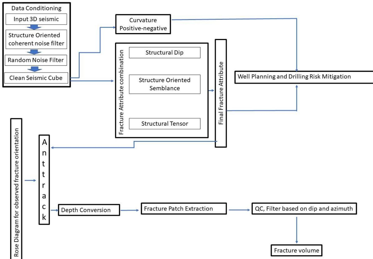
Figure 1. Workflow for seismic fracture characterization
