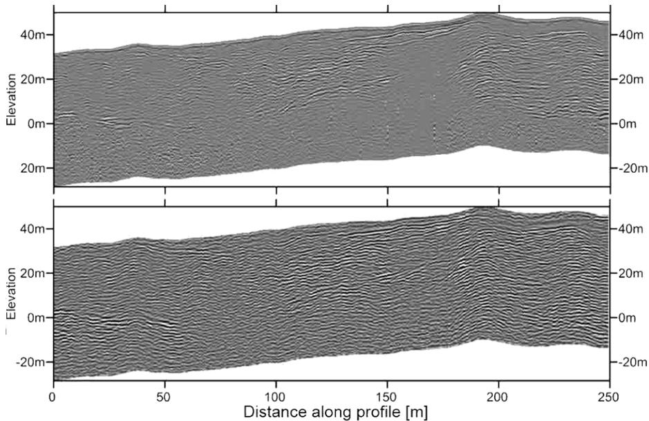
Figure 1 – Comparison of conventional GPR (top) and RTS UltraGPR (bottom) over sand dune showing significantly improved penetration
