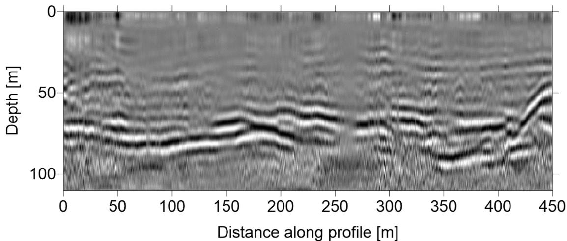
Figure 3 – Data from an RTS UltraGPR filtered to show only the 1 – 10 MHz bandwidth
