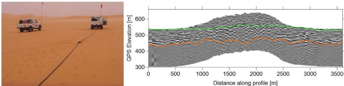
Figure 2 – 10 MHz RTS GPR being used for seismic static corrections in Libya to 200+ m (Francke, 2016)
