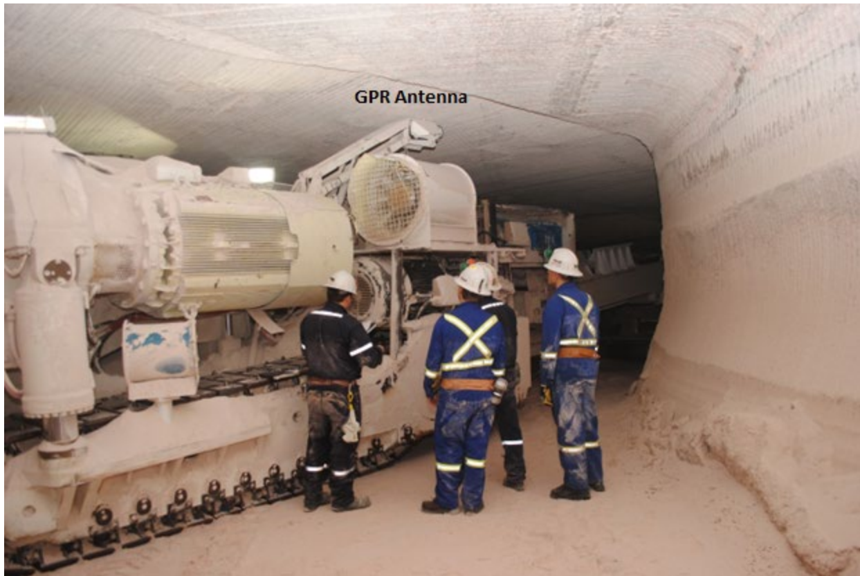
Figure 2: A prototype GPR unit being tested on a potash production boring machine at the Nutrien Cory potash mine. The GPR antenna is housed inside the box being held up against the roof by the retractable arm unit.
