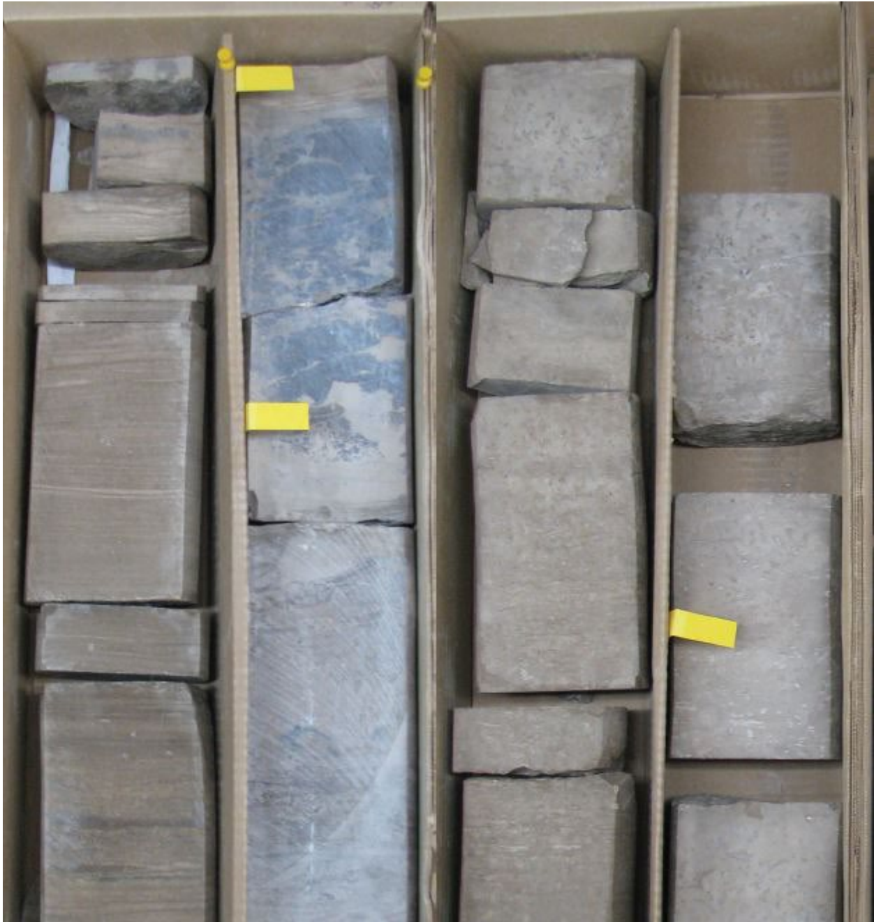
Figure 2. Interbedded porous recrystallized dolomite reservoir with tight anhydritic intervals in lower Beaverhill Lake pay
